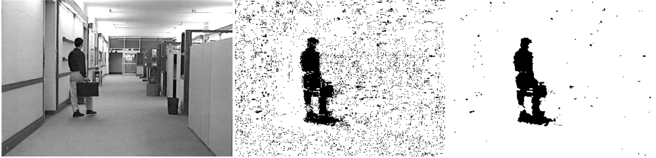
Fig. 2. Example of \Sigma\Delta processing. Left: original image of Hall sequence, middle: \Sigma\Delta without post-processing, right: \Sigma\Delta with 3 \times 3 morphological opening (erosion + dilation).
